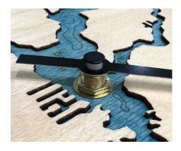
To remove the mechanism, first remove the center pin by pulling straight upwards. The tide hand is press-fitted to the shaft, so with gentle, even pressure at the base of the hand, pull up to remove it without damage. Now you will see the brass nut screwed to the shaft sitting on the brass washer. Use a 10-11mm deep socket, small wrench or a pair of pliers and unscrew the brass nut. The mechanism is now loose and can be removed from the back, along with the rubber washer.
